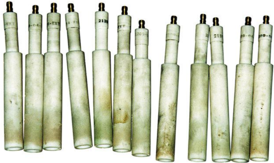
Plastic Extensions Fitted As Original Equipment By Dresser-Rand. After Less Than 1,500 Hours Of Operation
